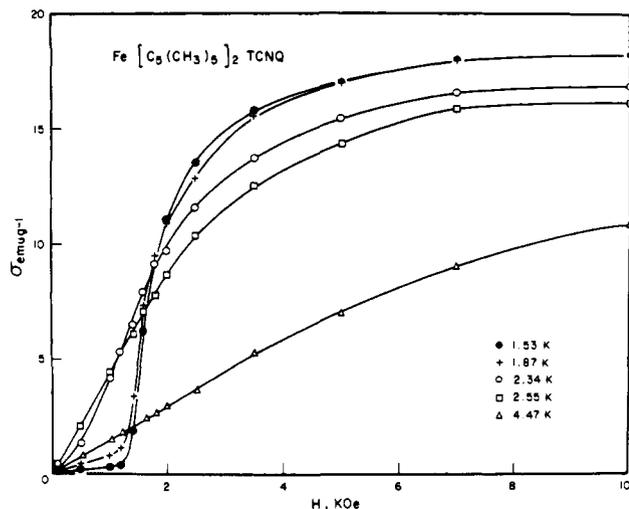
**Figure 2.** Isothermal plots of magnetic moment,  $\sigma$ , as a function of applied magnetic field,  $H$ . The sample is composed of small crystals of **2** as a pressed pellet.
