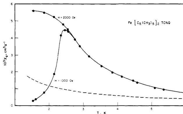
**Figure 1.** The magnetic susceptibility as a function of temperature between 1.5 and 6 K for **2**. The dashed line is the paramagnetism of the high temperature susceptibility extrapolated to lower temperatures. Complex **2** is antiferromagnetic below 1500 Oe and ferromagnetic above 1500 Oe.
